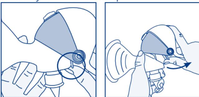
**Warning:** The handle (3) is the only component that never comes into contact with the milk; it is therefore sufficient to clean it with a soft cloth. If the handle is rinsed, dipped into water, cold sanitised with sterilising solutions, hot (steam) sanitised in sterilisers, or boiled this can prevent the product from working properly. It is highly recommended to maintain the handle periodically, following the instructions provided in the Handle Cleaning and Maintenance section.
