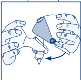
4. Screw the Step Up feeding bottle connector (6) onto the anatomical cup (2).
