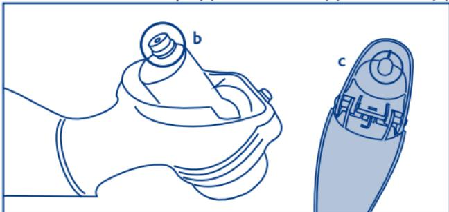
3. To assemble it correctly, apply light pressure downwards until you hear the handle flap click into place
