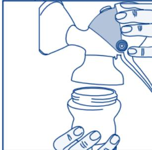
**2. Unscrew the Step Up feeding bottle coupling connector (6)**
