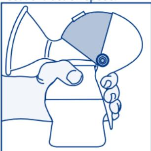
**Warning:** If the movement of the handle is difficult or insufficiently smooth, it is recommended to slightly oil the piston ring with some baby oil or similar product (to perform this operation, follow the instructions provided in the CLEANING, SANITISING & MAINTENANCE section. And Handle Cleaning & Maintenance section).
